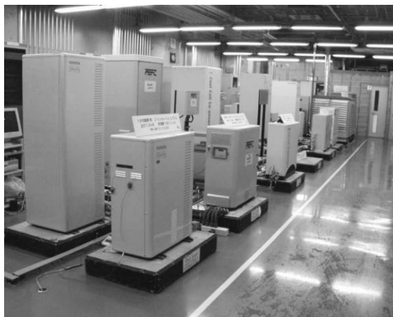
Fig. 8 1–5 kWe Residential fuel cell systems under evaluation in the Japanese Millennium Project. 117
